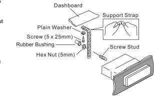
support. In these applications, place the rubber bushing over the screw stud and insert the radio.
